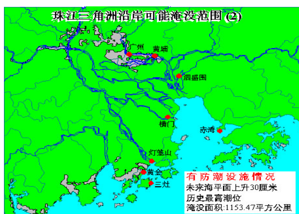
Figure 3.9 The possible submerged area by sea water under the scenario of sea level rise of 30 cm on the condition of the present tide-protecting facilities and the highest historic tidal level in the Pearl River Delta
